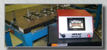
Stress relieving aluminum plates between rough and finish machining.
