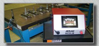
Meta-Lax Model 2400 stress relieving aluminum plates between rough and finish machining.
