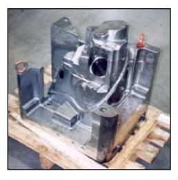
Specialty automotive headlight mirror-finished molds stress relieved with Meta-Lax have eliminated hardness cracking.
