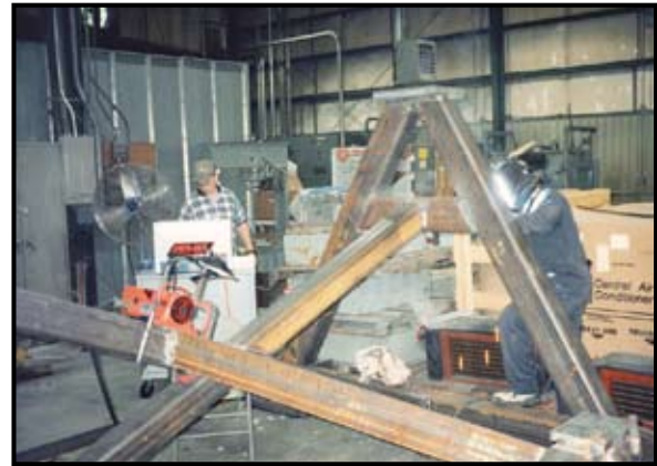
NASA’s Langley Research Center used Meta-Lax weld conditioning on a wind tunnel model balance calibration rig.
