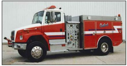
S&S's newest Meta-Lax treated off-road fire truck, the "Outback." Designed for wildland fire fighting, the Outback allows 3,000 lbs. of equipment and hose capacity with a full tank of water, cab space for three and a 1,000 lb. reserve.
