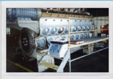
16-Cylinder Diesel Marine Engine
