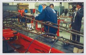
**Chassis Being Weld Conditioned**
