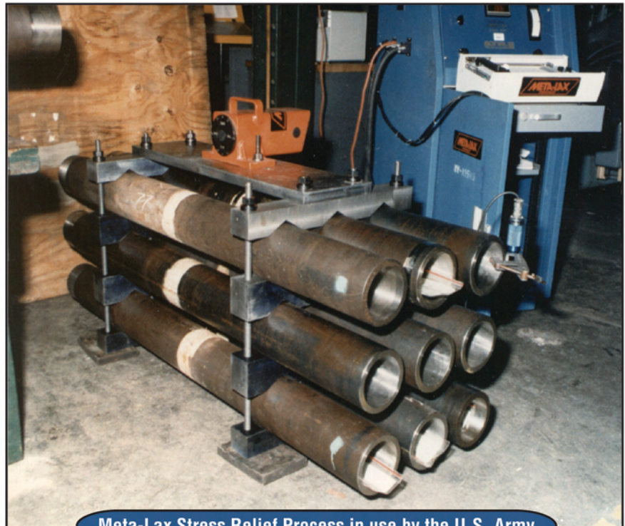
Meta-Lax Stress Relief Process in use by the U.S. Army
