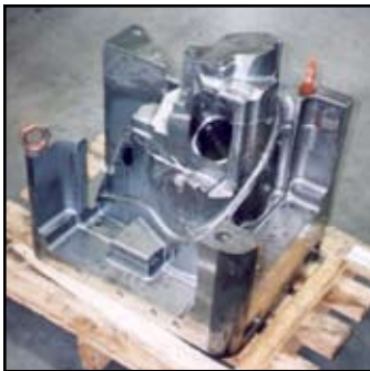
A heat treater's nightmare due to extreme differential thicknesses.
