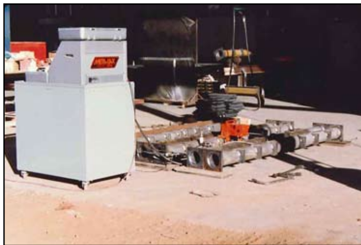
Corrosion Engineering uses Meta-Lax to stress relieve these cross-tubes saving approximately $70,000 over thermal stress relief.
