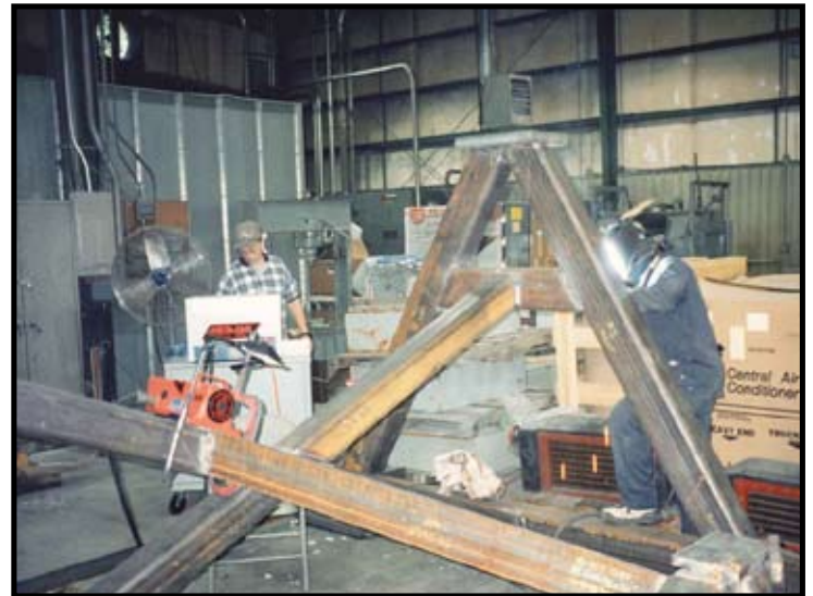
NASA's Langley Research Center uses Meta-Lax weld conditioning on a wind tunnel model balance calibration rig.
