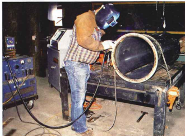
Using sub-harmonic vibrations at the time weld repairs are made has significantly shortened turn-around time for a West Virginia testing and repair facility.
