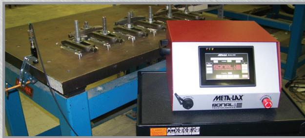
Stress relieving aluminum plates between rough and finish machining.
