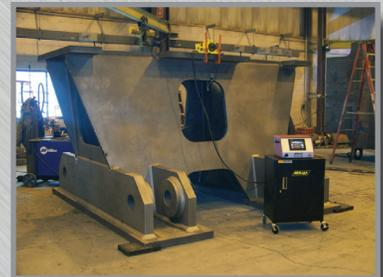
Meta-Lax Model 2400 stress relieving 50,000 lb low carbon steel weldment after welding before machining.
