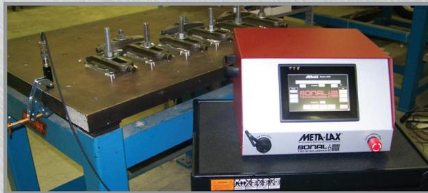
Meta-Lax Model 2400 stress relieving aluminum plates between rough and finish machining.
