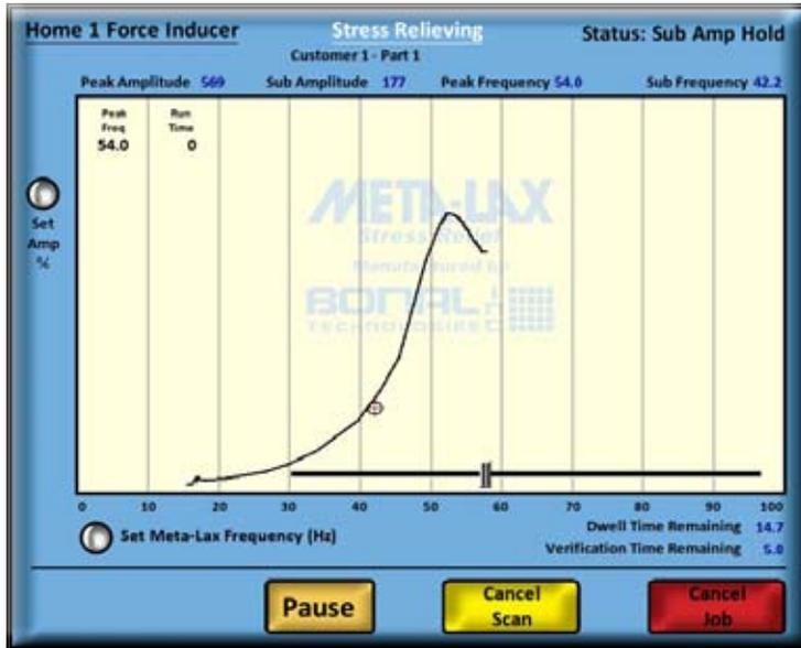
The entire stress relief and or weld conditioning procedure is completed directly from this screen.
