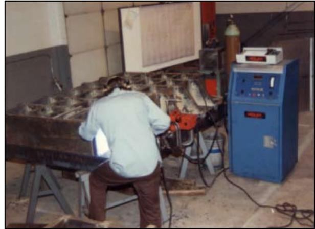
**A 10,000 lbs. platen, Meta-Lax Weld Conditioning reduced severe weld cracking.**
