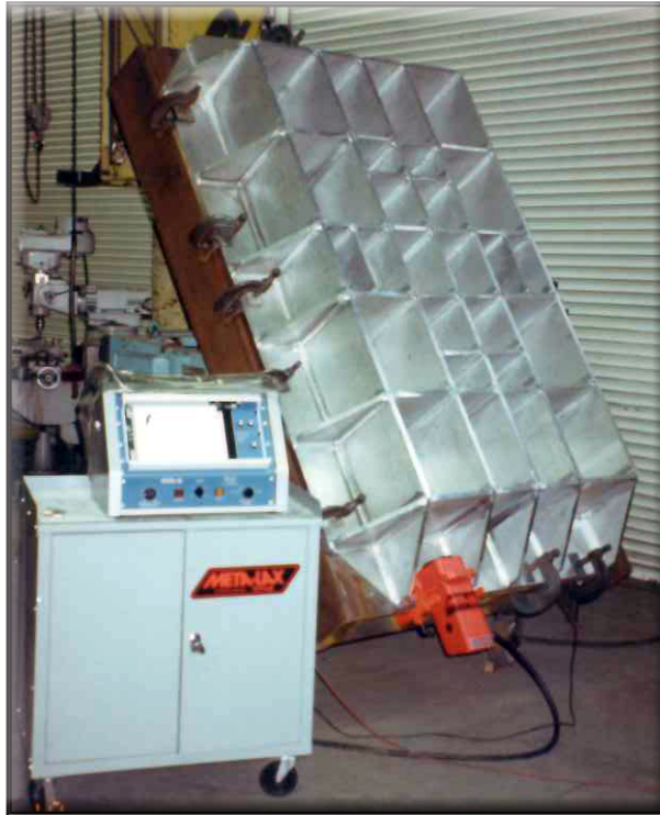
This honey comb platen was Meta-Lax weld conditioned and obtained 90% better than normal distortion.
