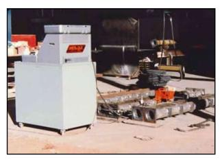
Corrosion Engineering uses Meta-Lax to stress relieve these cross-tubes saving approximately \$70,000 over thermal stress relief.
