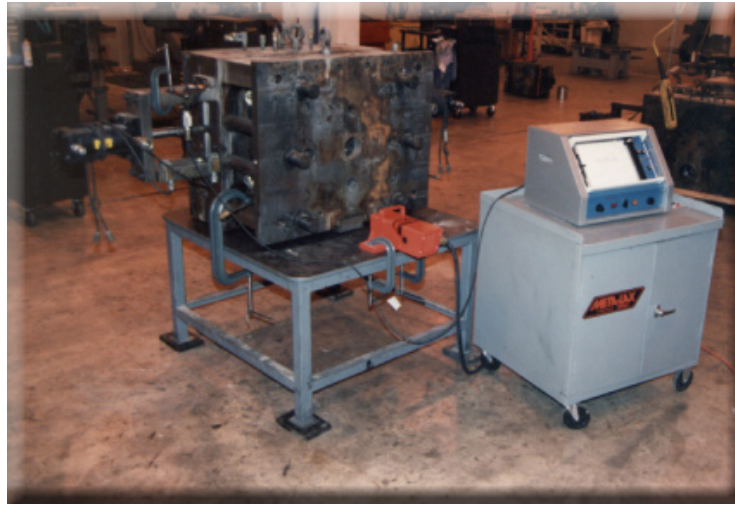
Assembled die casting die being Meta-Lax treated.
