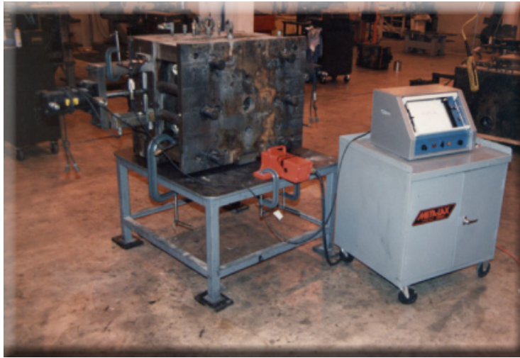
Assembled die casting die being Meta-Lax treated.
