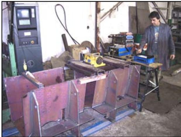
***Metalonica makes many custom weldments which are now Meta-Lax stress relieved in-house to save time and money as well as to maintain high quality. This weldment was Meta-Lax treated to assure that it will hold proper alignment in service.***
