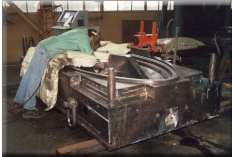
After nearly 80 hours of using Meta-Lax during welding at Modern Tooling Systems, no cracks or porosity were detected.
