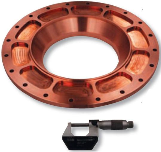
***Prior to using the stress-relief system, copper injector plates, with 14" diameters and a 1/2" flange on top, were out of flatness by 0.005". After use of the Black Magic system, distortion after machining was reduced by 80 percent.***
