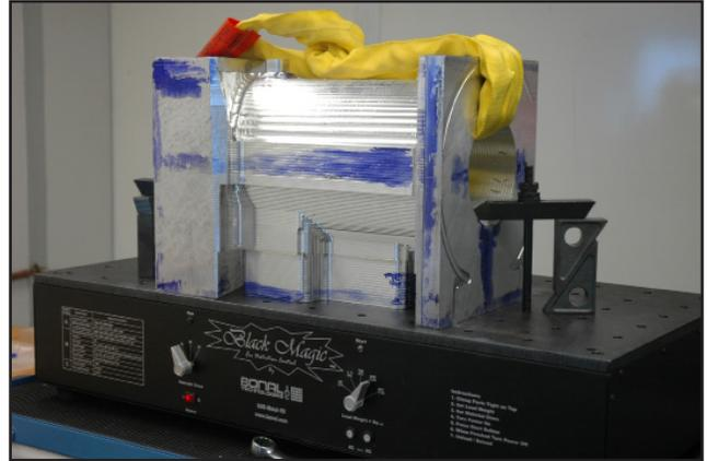
**Relieving stress in parts before machining results in less distortion. By mounting pieces on the Black Magic stage and subjecting them to sub-harmonic vibration, Mooney Industries reduced parts warpage and reworking.**
