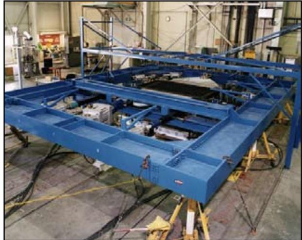
**Setting Up-Shop specialists at the NASA Dryden Flight Research Center prepare the new test assembly fabricated there for a lengthy series of load and thermal tests on the titanium matrix composite panel already positioned inside the 12 ton "I" beam assembly. The test article is a side shear fuselage panel demonstrating aerospace plane technology.**
