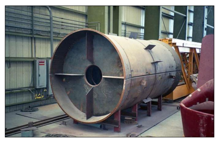
This drum material would normally be welded using 300°F preheat. To preheat this drum would have made it extremely dangerous to weld the inside. Meta-Lax weld conditioning was used instead of preheat. No problems occurred in welding.
