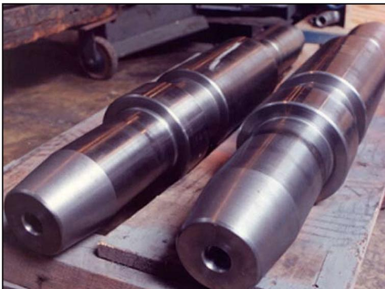
*These 8620 grinder spindles, 4-in dia. x 36-in. are Meta-Lax treated to reduce distortion 80% to 10 millionths of an inch.*
