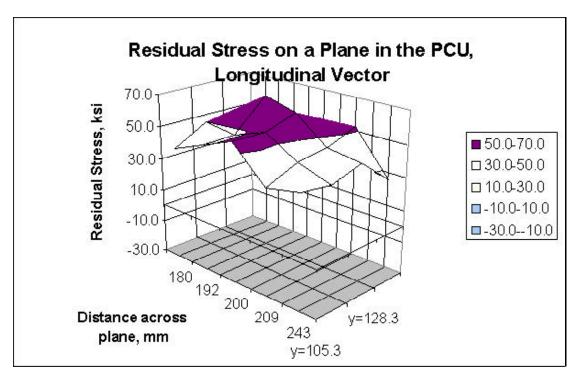
Above, neutron defraction through center of cast aluminum aircraft part. Approximate average residual stress level = 45,000 psi.
