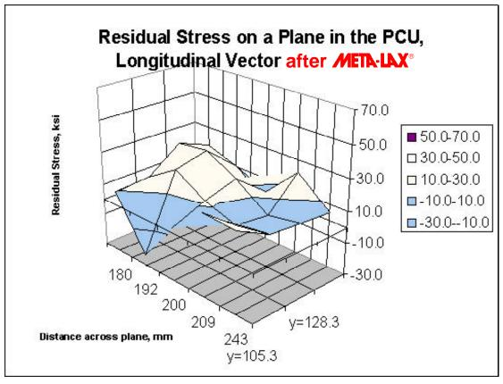
Above, same component retested after Meta-Lax (Sub-Harmonic Vibration) stress relief treatment by Bonal Technologies, Inc. Approximate average residual stress level = 0.
