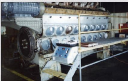
**16-Cylinder Diesel Marine Engine**
