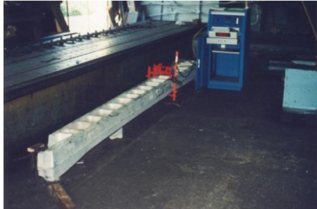
Normal Performance. Normal distortion always exceeded tolerance to the point that special approval was given to accept longerons with an overall distortion that was less than 0.200-inch. Even with the special approval, scrap rate was around 90 percent.
